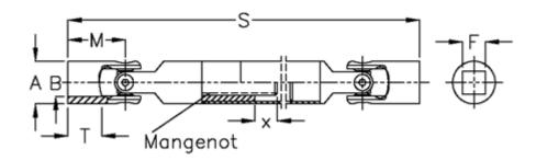
A = 32 F = 16 Longitudinal ribs = 6x16x20M = 43 MD max N m = 40 s = 234T = 25x = 30
